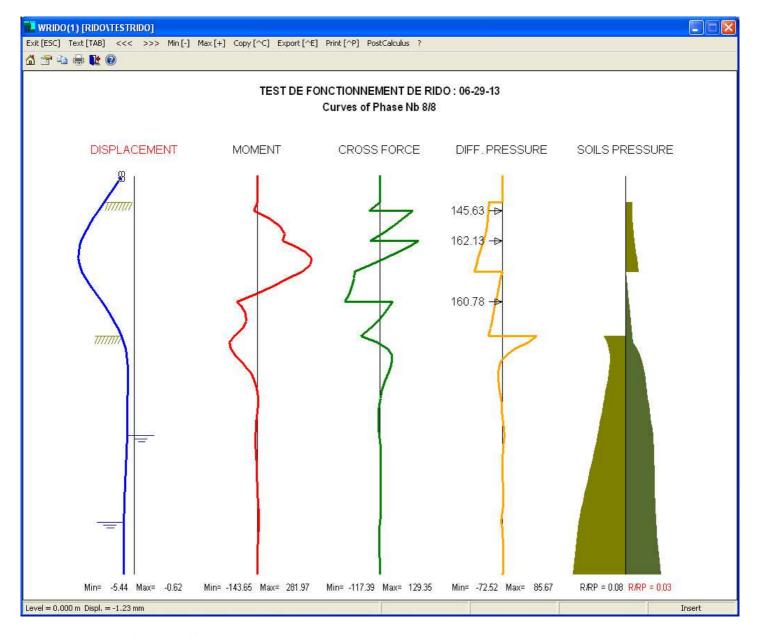
We can here visualize the different results curves for all the phases with the same scale, and also the envelop curves.
