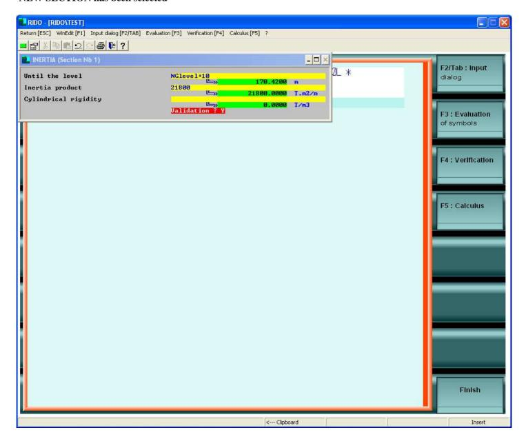
On a 12 meters height, the inertia of this section of retaining wall will be 21800 T.m2/m
