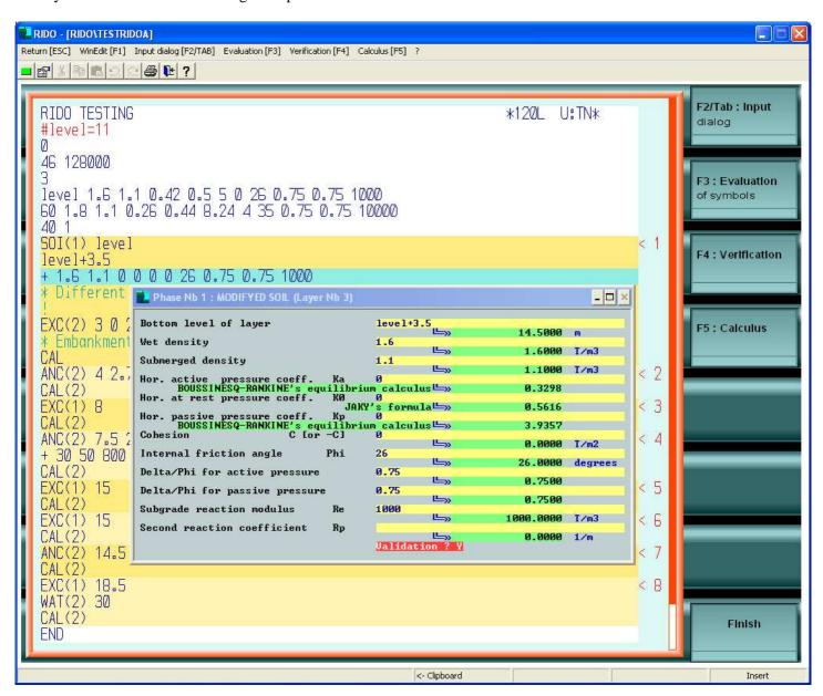
It's important to notice that the evaluation of the coefficients Ka and Kp is done by resolving the differential equations of Boussinesq-Rankine and that the evaluation of the coefficient K0 is done by using the Jaky formula.
